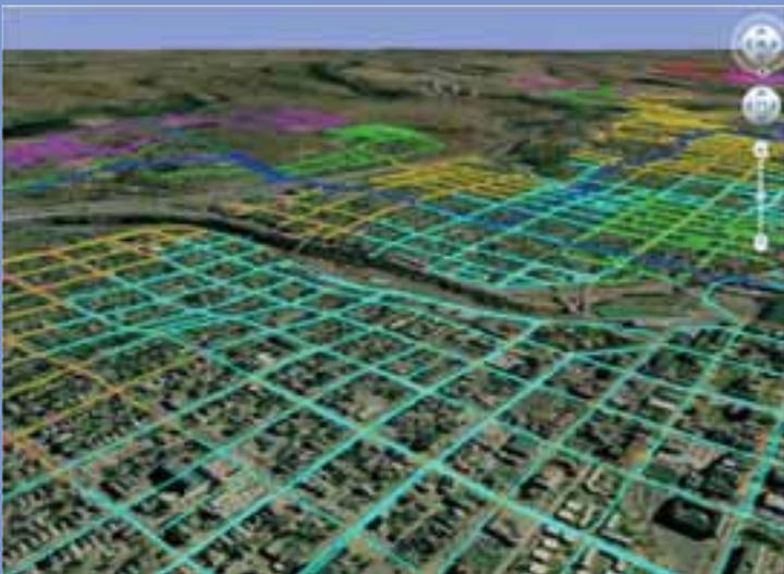
Figure 3: Water pipe network from WaterGEMS software exported to Google Earth™
