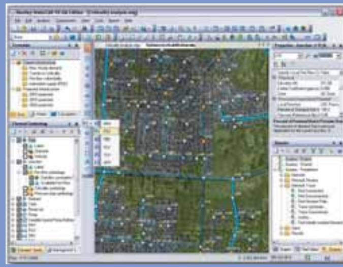
Figure 2: Finding critical pipes and valves to prioritize rehabilitation investment
