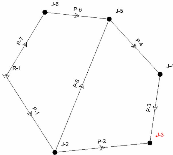
Figure 4 A sample system with the nodal reference pressure head of 40 meters and threshold pressure of 65.0 meters
