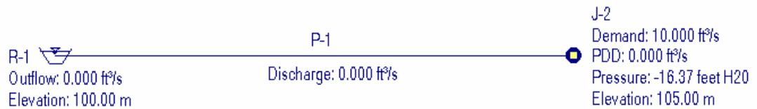
Figure 2(c) Calculated PDD is zero due to the pressure is negative.
