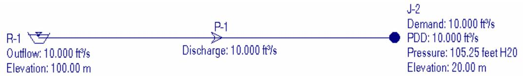
Figure 2(a) Calculated PDD is the same as demand due to the pressure is above the pressure threshold.
