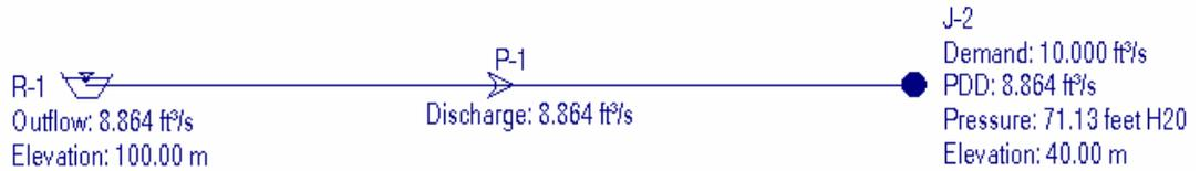
Figure 2(b) Calculated PDD is less than the required demand due to the pressure is lower than the pressure threshold.
