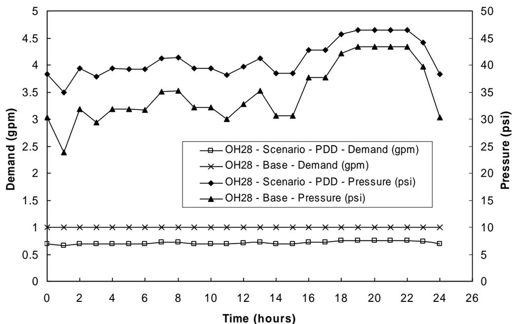
Figure 7 Comparison of the simulated demand by conventional model and pressure dependent demand model when emergence operation occurs at OH24
