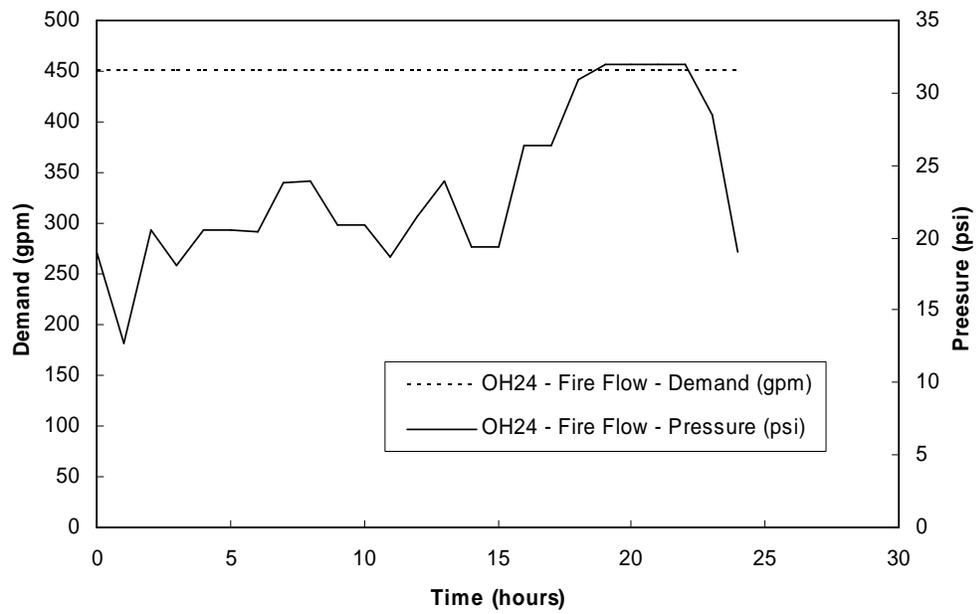
Figure 6 Calculated pressure and demand when a big user constantly draining water at node OH24 out of the system
