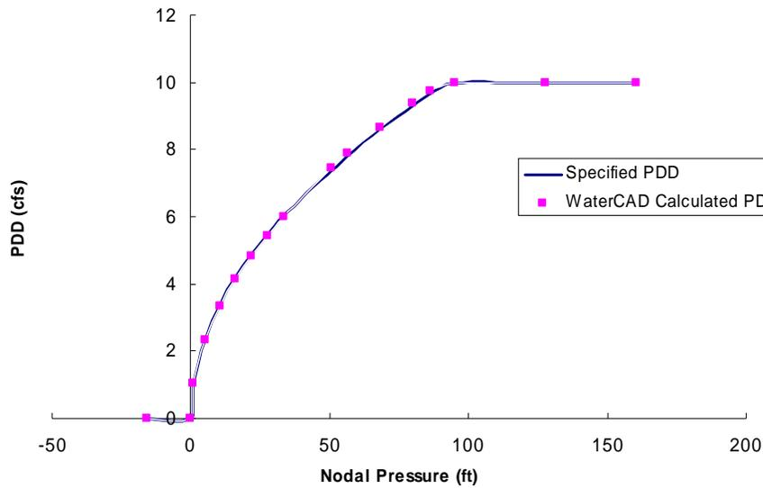
Figure 3 Comparison of the calculated PDD with specified PDD for exponent of 0.5
