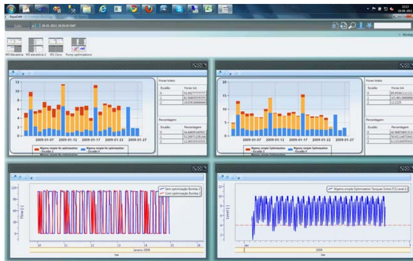
Figure 8 – Alternative scenario analysis by reprogramming pumping periods. At the top, the left image shows the present regime and the right image shows an alternative. Below, one may see pump functioning periods and reservoir levels.
